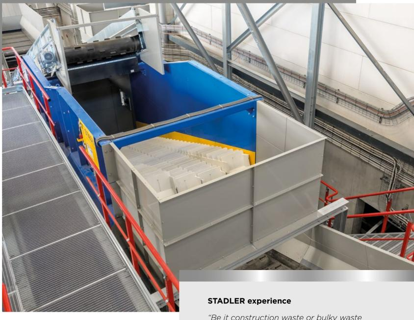
Thanks to our ballistic separator STT6000, even large and heavy objects can be separated into flat and rolling fractions without difficulty.
