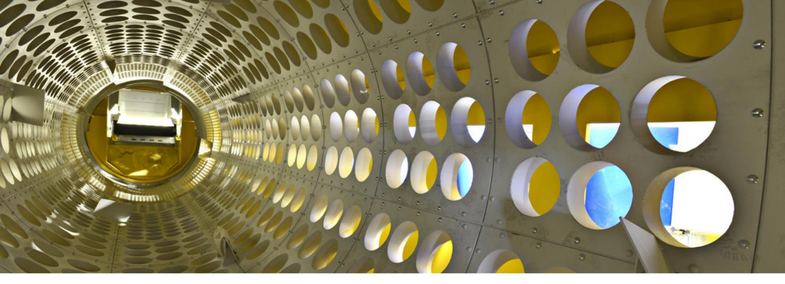
STADLER screening drums are characterized by their exceptional robustness. They are manufactured from 10 millimetre-thick steel (e.g. hardox) and are highly torsion-resistant. They are equipped with spacious walkways, draw bridges and doors as well as interior lighting, which makes them especially easy to maintain.
